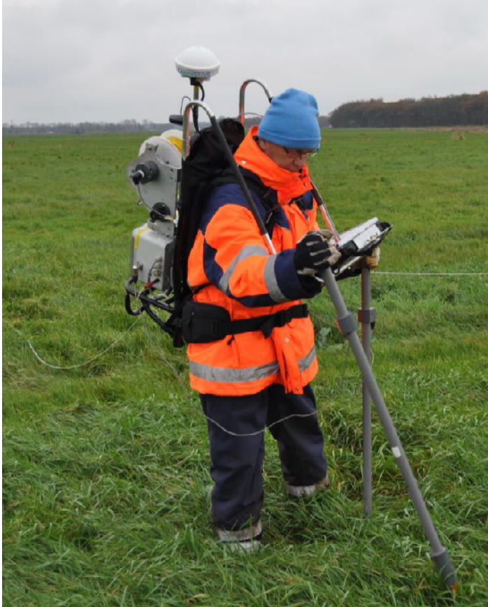
Figure 8: The Cathodic Protection Survey Set
